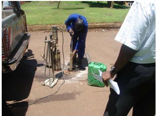
Picture 12: Coring to test asphalt quality on Philip Road. Spenco/PROME
